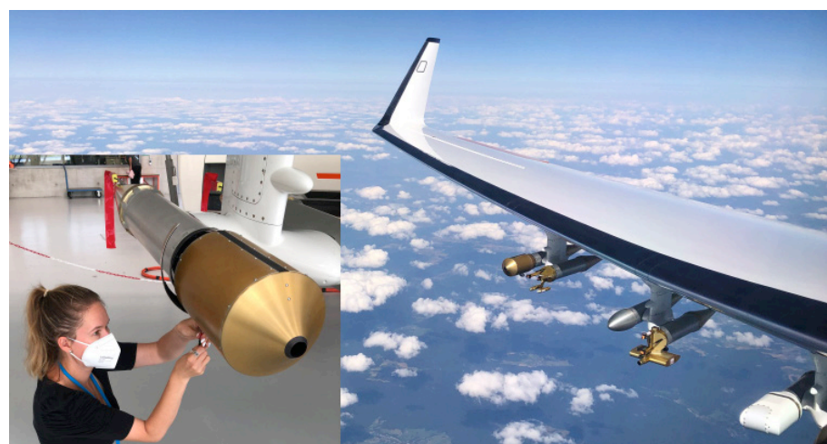
Particle Habit Imaging and Polar Scattering probe attached to a wing of the research plane HALO. (Photo: Emma Järvinen, KIT)
